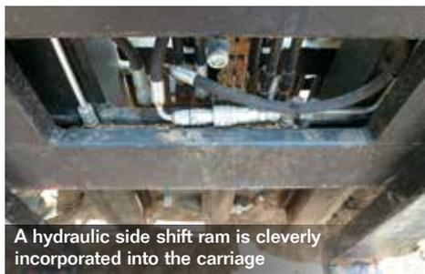
A hydraulic side shift ram is cleverly incorporated into the carriage
