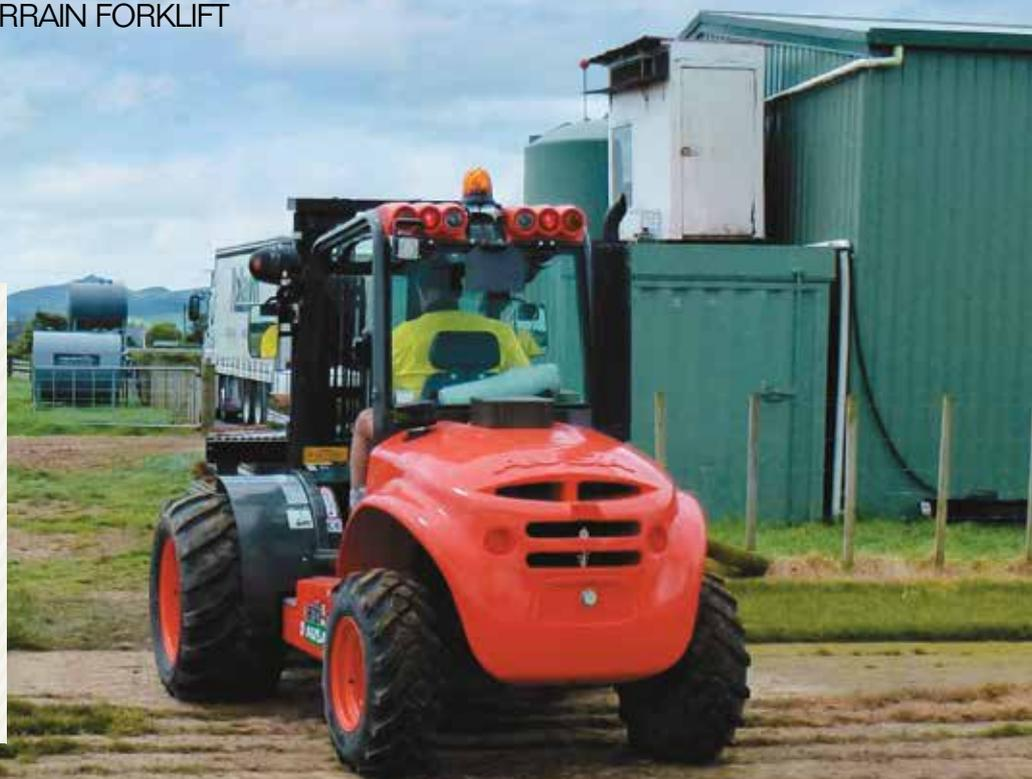
A large rounded counterweight on the back protects the engine and balances the forklift
