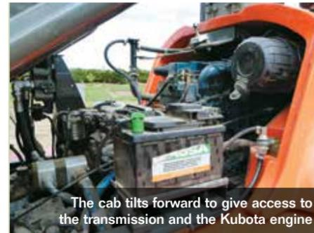
The cab tilts forward to give access to the transmission and the Kubota engine
