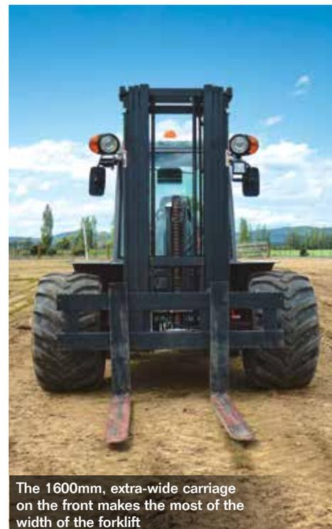
The 1600mm, extra-wide carriage on the front makes the most of the width of the forklift
