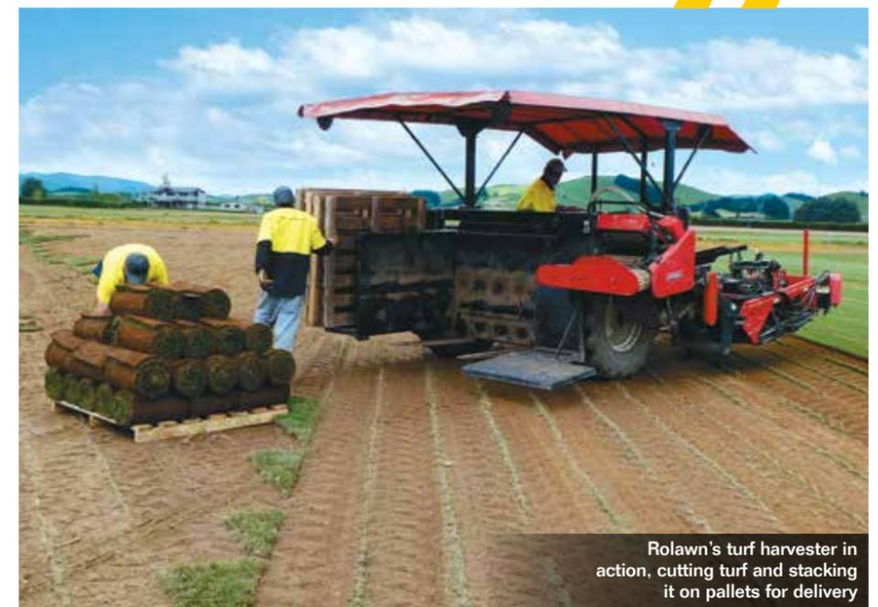
Rolawn's turf harvester in action, cutting turf and stacking it on pallets for delivery
